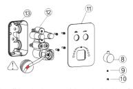
Take off the plastic cover of the embedded box® with a screw driver, fix the shower valve@on the embedded box®with screw , install the panel ® and handle ®, install the valve screw®into the handle, and finally install the handle cap®.
