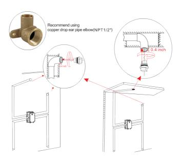
1:Recommend using Copper drop ear pipe elbow(NPT 1/2 ) USA:1/14 NPT 2 -Canada:1/2"-14 NPT Europe:G1/2"
