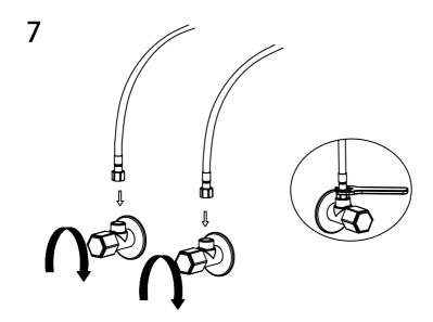
7. Connect the hot & cold supply lines onto the matching water valves and secure the connection with an adjustable wrench.
