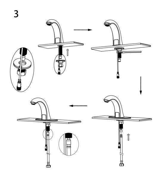
3. Slide the metal washer first.and then the spanner tighten and mounting nut.finally connect faucet with flexible pipe.
