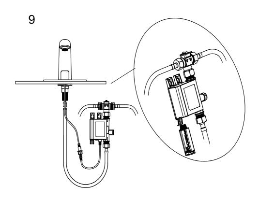
9. Remove the battery pack cover and take out the battery pack; insert 2 AAA batteries. put the battery pack back in the control box and replace the cover firmly.
