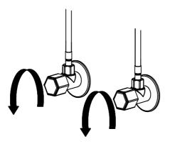
10. When install ation steps 1-10 are completed, turn the hot & cold water inlets back on.
