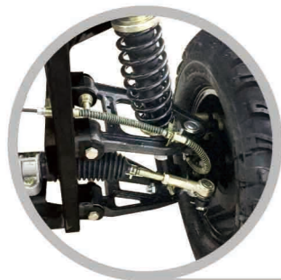
Premium Comfort Suspension Independent Front Suspension with Double Arm
