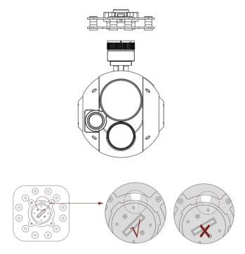
1. Make sure the two white stripes indicated in above picture are aligned with each other. (If the stripes are not aligned to each other, please pinch the connector part and turn it to left manually)
