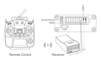
Wiring Diagram Standard Version
