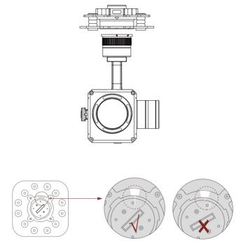
1. Make sure the two white stripes indicated in above picture are aligned with each other. (If the stripes are not aligned to each other, please pinch the connector part and turn it to left manually)
