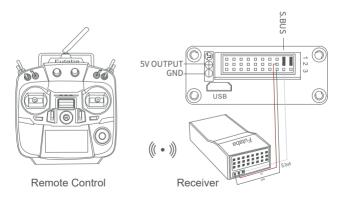
Wiring Diagram Standard Version
