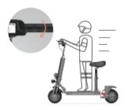
3. Turn the knob to open the accelerator and start riding Slow down by releasing the throttle
