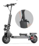
5. Install the seat bag and fix the folding buckle
