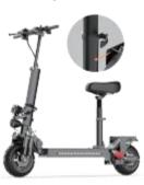
2. Straighten the frame and fixthe buckle
