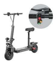
6. L and H two gear speeds, yellow button for left and right adjustment, Green button switch horn
