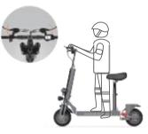
4. Gently hold the brake handle to slow down, Hold the brake handle tightly for emergency braking
