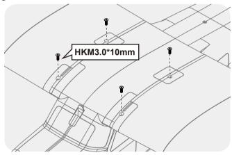
${\it 4.A lign the holes of support bars with the holes on the fuse lage and the main wing.}\\$
