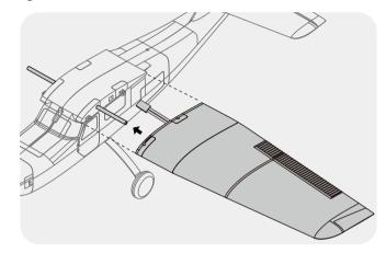
3.Use the included screws to secure the wing halves to the fuselage.
