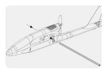
2. Apply the left and right wing halves onto wing spar, pass the servo wires into fuselage and then have them connected with a 2Y harness.
